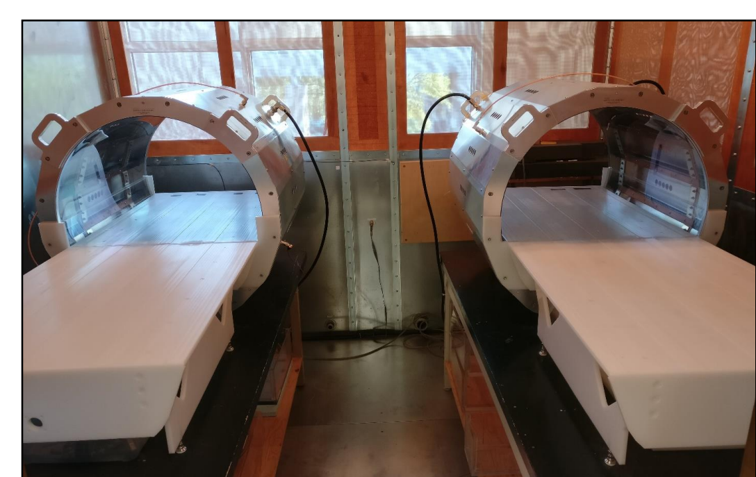
Figure 1: MITS 1.5/64 MHz (left) and 3.0/128 MHz (right) bench top exposure systems [2].
